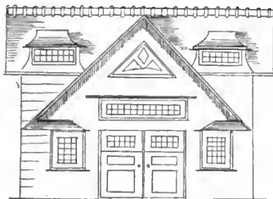
FIG. 1.—Stable front altered for transformation into a garage.
